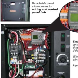
**Smart Relay Control** provides complete control over run time, auto start/stop and time delay shut down functionality.
