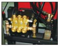
**Large frame Hotsy belt-drive pump** features NESTechnology with U-Seals for 3 times longer pump life.
