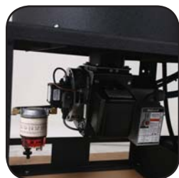
Beckett burner with fuel/water separator
